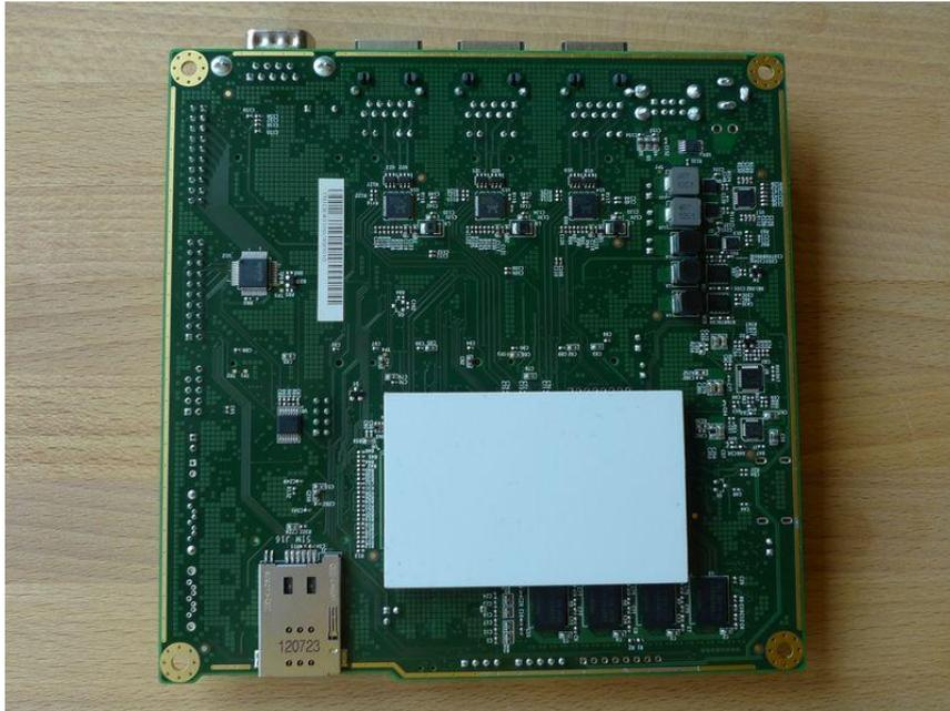
3. "Bottoms up" - hold the enclosure base upside down, feed the board DB9 and LAN connectors through the openings. Lightly press board and enclosure base together to stick the heat spreader in place.
