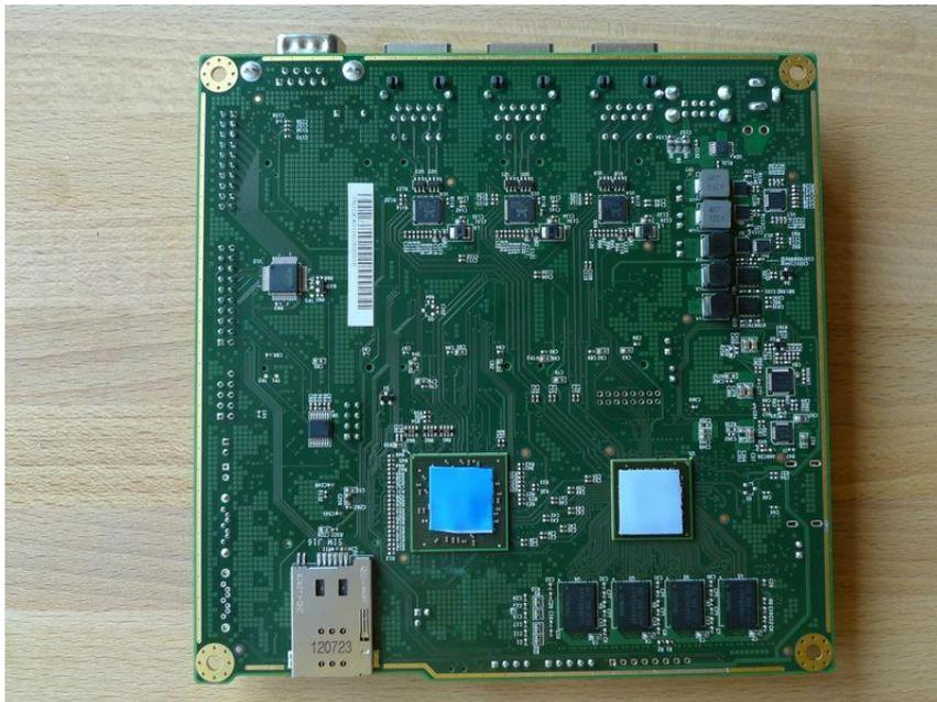
2. Place the aluminum heat spreader (blank side down) over CPU and south bridge. Make sure to avoid conflict with nearby through hole components. Peel the cover foil.
